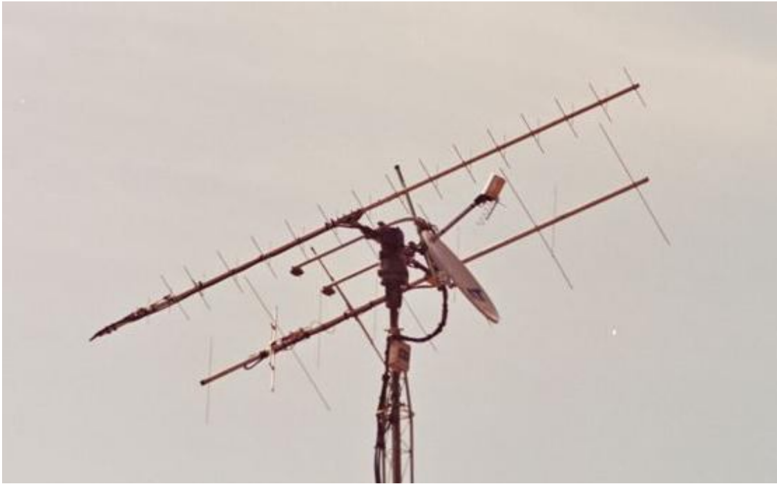
Side view of a typical aerial system of a base station for amateur satellites
